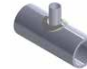
Reinforcement Pad Perpendicular
